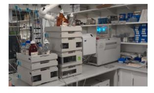
Pictured: Agilent 1100 HCT ion trap Protein digests.
