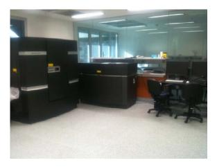
Pictured above: OMX Blaze, 3D structured illumination microscope. This super resolution microscope permits imaging below the diffraction limit with resolutions typically of 90-130 nm in x,y and 250-350 nm in z It is equipped with
